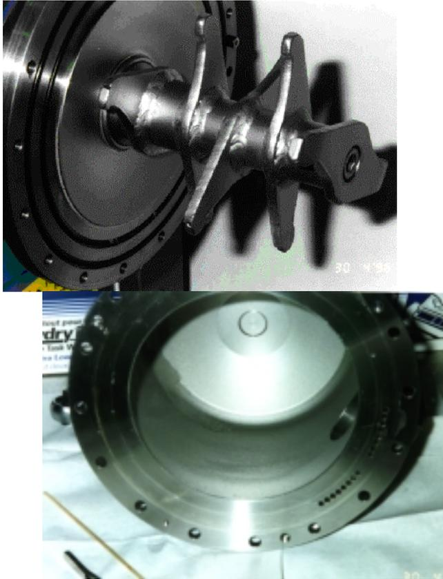
*Fig. 11.a+b: Grinding chamber after cycle operation ( $\text{Fe}_3\text{Al}$ , Oak Ridge National Laboratory, Oak Ridge, TN)*
