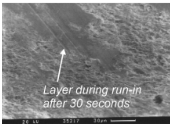
Fig. 14.a: SEM-micrograph of the surface of a powder pellet after 30 seconds (Fe-40(MoS 2 ), 10 hours of MA)
