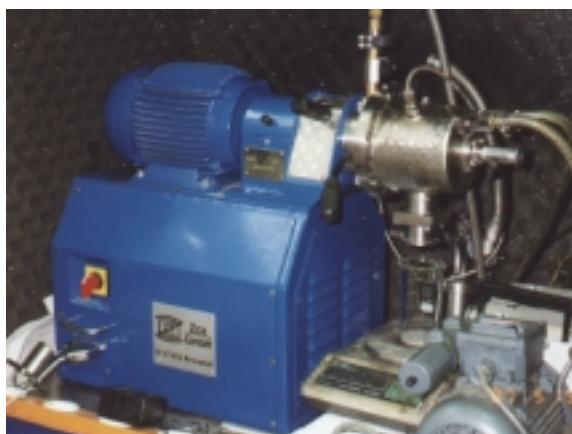
Fig. 4.a: Simoloyer CM01 used for powder processing
