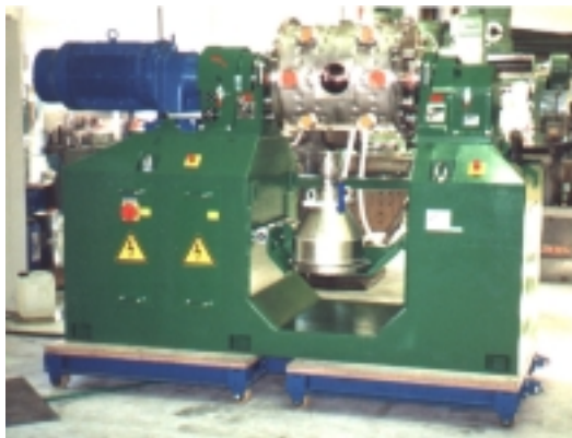
Fig. 1: Simoloyer ® CM100s, 100 l capacity for semi-continuous powder processing
