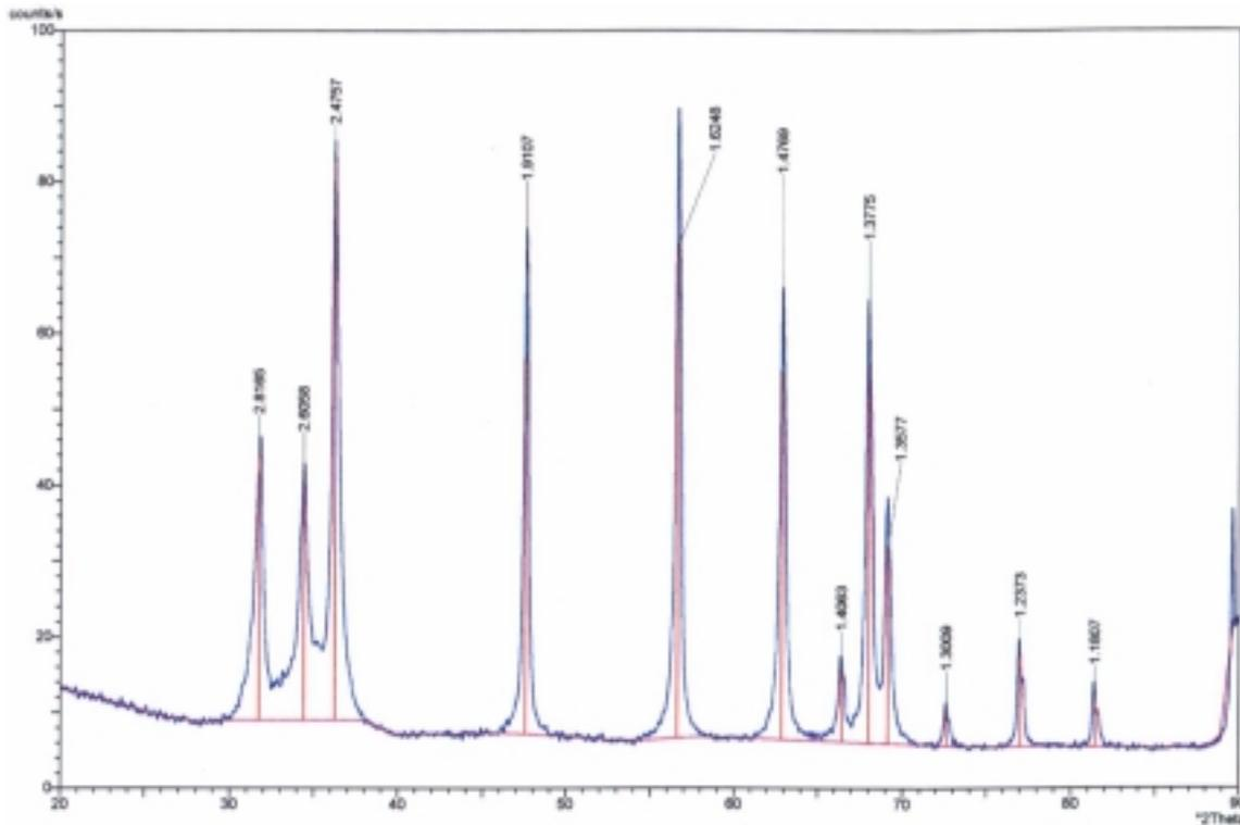
Fig. 7: XRD-analysis of ZnO, starting powder
