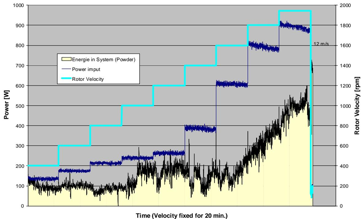
Fig. 4: Measured Powder Energy
