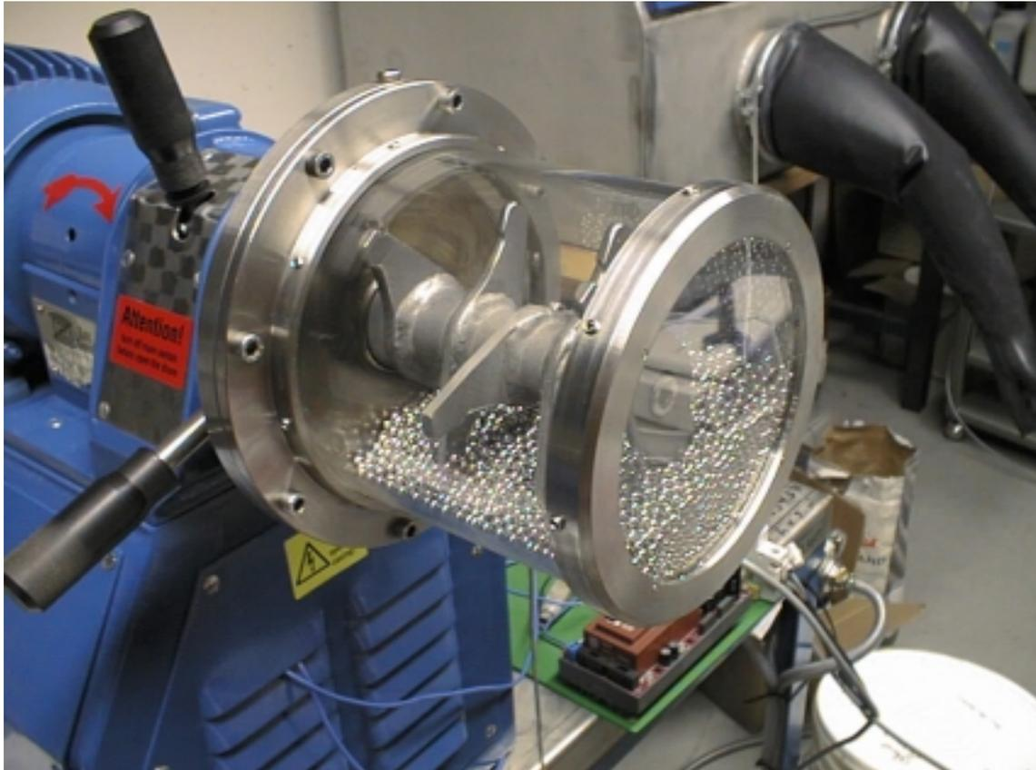
*Fig. 5: Transparent 2 liter grinding unit connected to laboratory scale mill Simoloyer<sup>®</sup> CM01*
