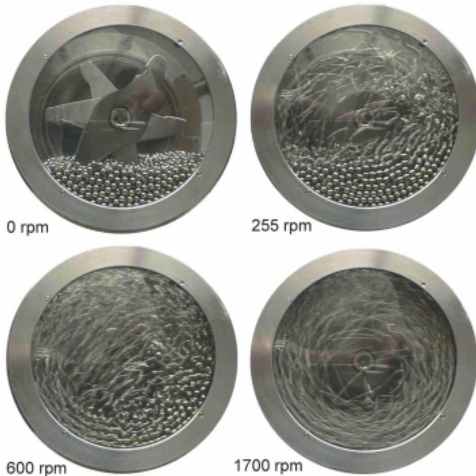
Fig. 6: Grinding media motion while operation
