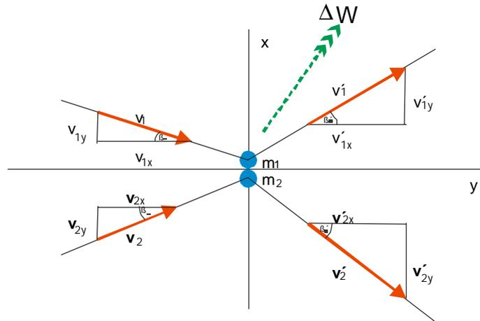
Fig. 2: Collision of grinding media
