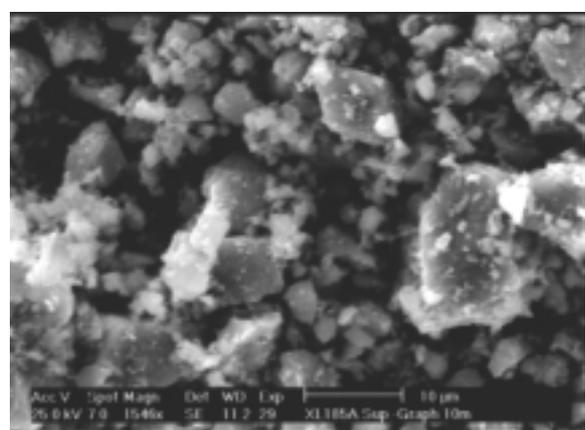
*Fig. 14b: Particle sizes of SiC powder after 10min*
