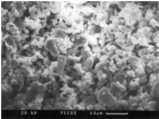
*Fig. 15a: Particle sizes of  $\text{Al}_2\text{O}_3$  starting powder*
