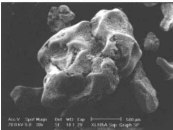
*Fig. 14a: Particle sizes of SiC starting powder*
