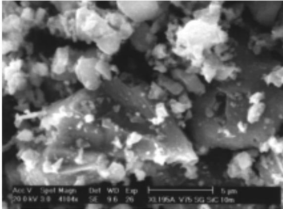
*Fig. 14c: Particle sizes of SiC powder after 10min processing*
