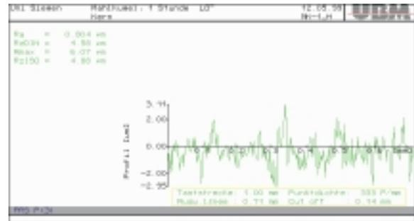
Fig. 11b: Roughness measurement after 14h
