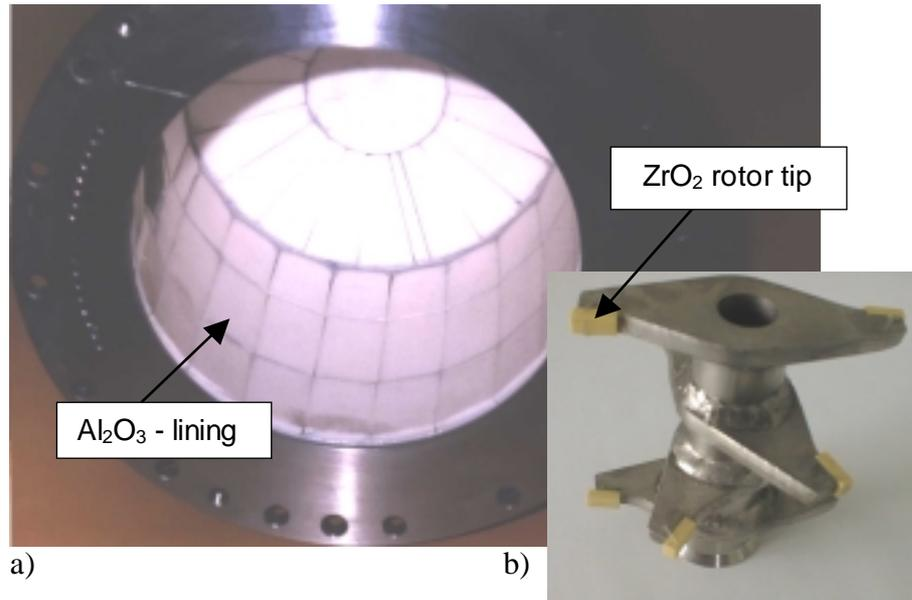
Fig. 4: Grinding parts of prototype 3
