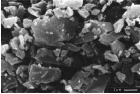
*Fig. 16a: Particle sizes of quartz starting powder*
