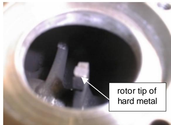
Fig. 8: Hard metal rotor after 20h:
