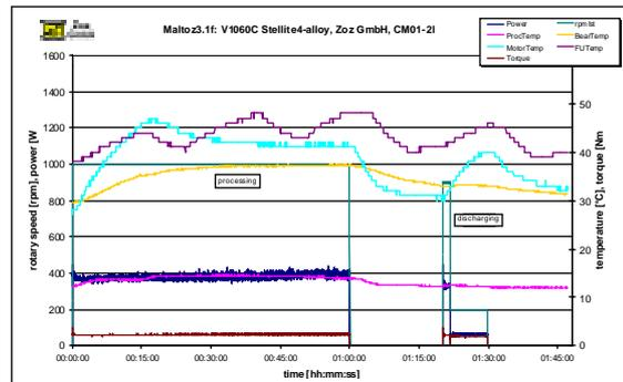
In case of processing pure stellite-material as well as alloying element A, constant operation has been suitable, in case of alloying element B, Cycle Operation [16, 17] has been applied in order to avoid agglomeration during processing.
