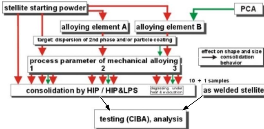
Fig. 18: flow-chart of powder production by HKP for the consolidation of 10 different samples
