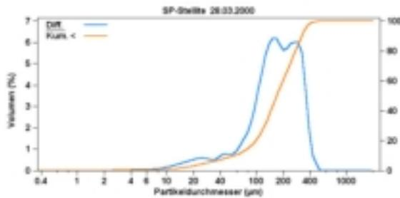
*Fig. 20: particle size distribution*
