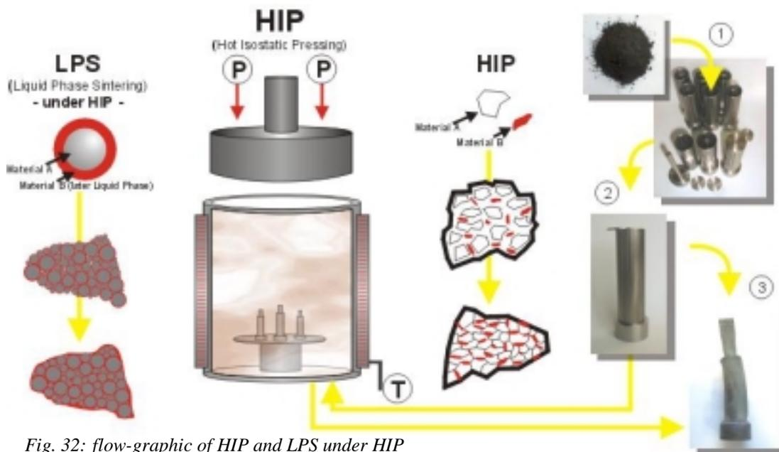
Fig. 32: flow-graphic of HIP and LPS under HIP
