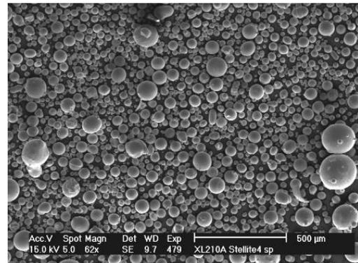
*Fig. 21: SEM of stellite starting powder*
