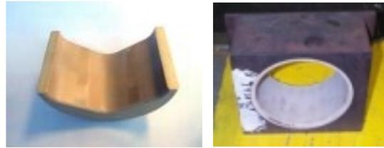
*Fig. 11: sintered zirconia bearing components*
