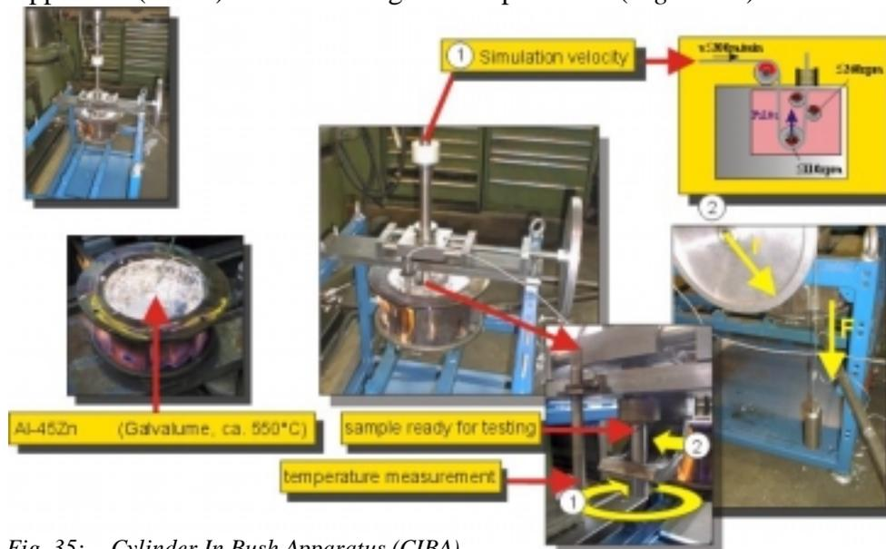
*Fig. 35: Cylinder In Bush Apparatus (CIBA)*
