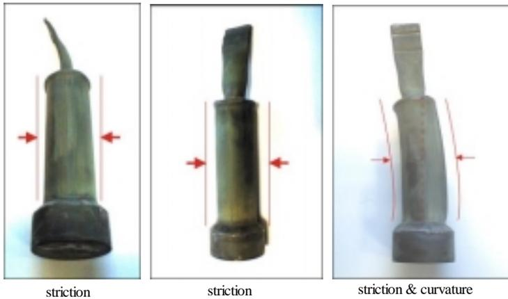
*Fig. 33: deformation behavior during consolidation by HIP and LPS under HIP*
