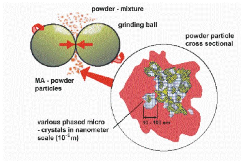
Fig. 13: schematic of collision, principle of HKP
