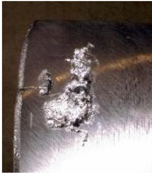
The PM-consolidation route is considered to be certainly superior to casting and welding due to a unique bulk-structure and a full dense material. Inclusions and hollows (*Figure 14*) in the bearing material will not any longer be present at all. In particular cracks and micro-cracks cause major losses as they act as a diffusion speedway for the liquid metal. This is avoided by the application of HIP for consolidation.
