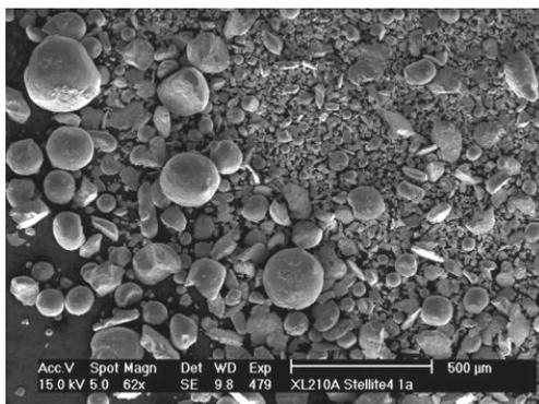
*Fig. 22: SEM of PM09MA1A*
