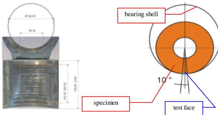
Fig. 36: used counter-bearing of galvanizing plant, determination of reference area
