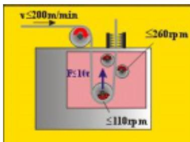
Fig. 04: transfer system inside the crucible of a hot-dip galvanizing/aluminizing plant
