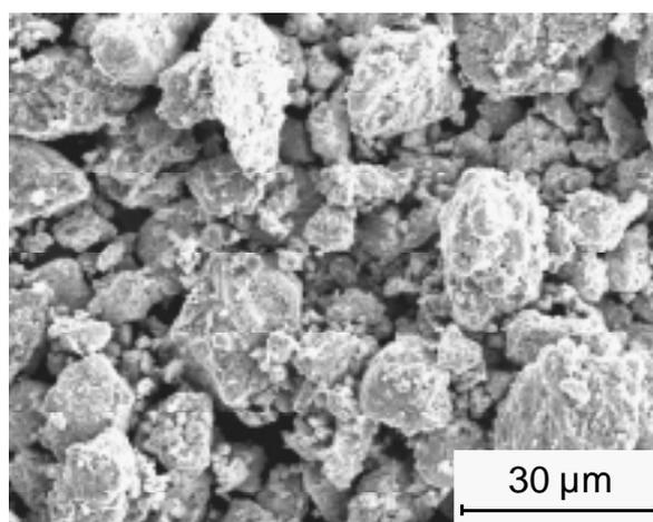
**Figure 2.** Morphology of the mechanically alloyed composite particles.
