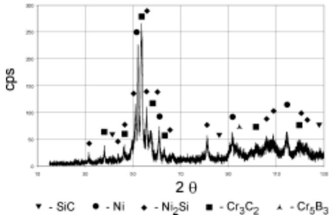
**Figure 8.** XRD pattern of a Ni-based nano-structured SiC composite coating, SiC content in the composite powder: 65 vol.-%, Top Gun K.
