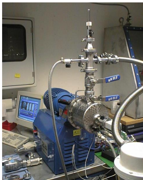
Figure 1: 2-L horizontal high energy ball-mill (Simoloyer® CM01-2l) with vacuum and inert-gas loading, operation and unloading.
