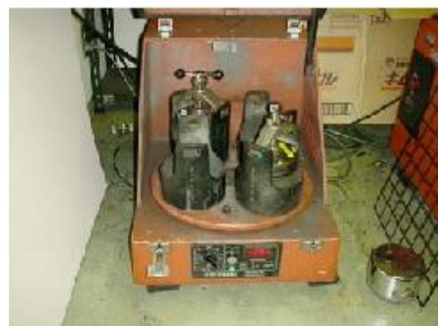
Figure 3b: planetary ballmill Fritsch P-5
