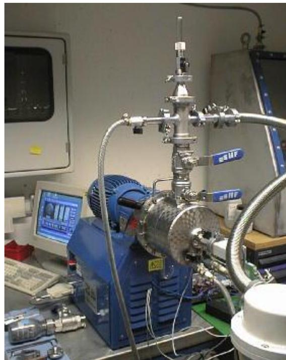
Figure 5b: horizontal high energy ballmill (Simoloyer CM01-2l) with air-lock for loading, operation and unloading under vacuum and/or inert-gas
