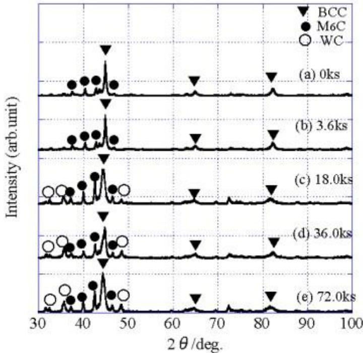
Figure 16: XRD-pattern of SPS-samples consolidated from the MM-powder after 0, 3.6, 16, 36 and 72 ks at high kinetic (CM01)
