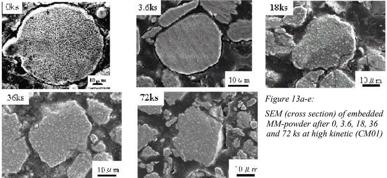
Figure 13a-e: SEM (cross section) of embedded MM-powder after 0, 3.6, 18, 36 and 72 ks at high kinetic (CM01)
