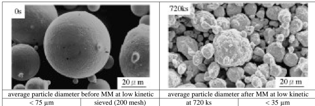
Figure 10: SEM of MM-powder after 0 and 720 ks at low kinetic (PBM)
