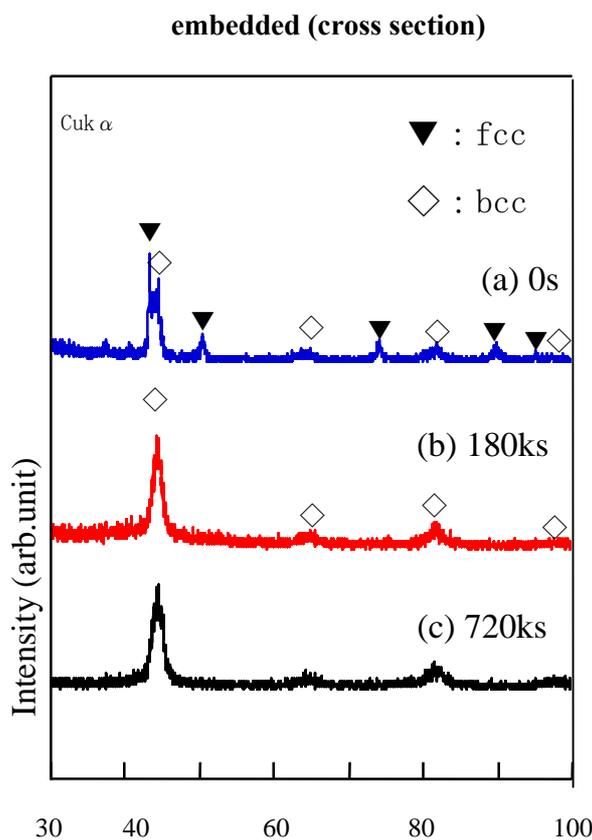
Figure 12: XRD-pattern (cross section) of embedded MM-powder after 0, 180 and 720 ks at low kinetic (PBM)
