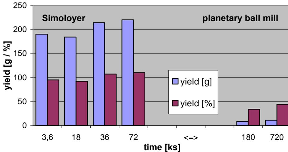
Figure 8: powder yield results & processing time after high- and low kinetic MM
