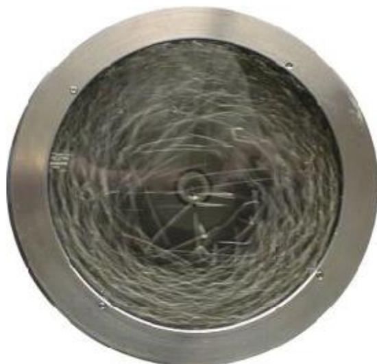
Figure 5a: collision effects in high-kinetic MM (Simoloyer)
