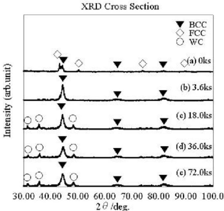
Figure 14: XRD-pattern (cross section) of embedded MM-powder after 0, 3.6, 18, 36 and 72 ks at high kinetic (CM01)
