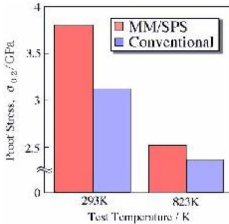
Figure 18: Proof stress of conventional HSS-compact by HIP/Forging and of MM/SPS compact
