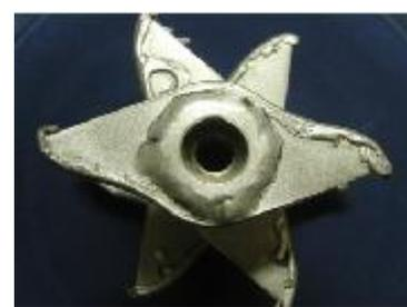
completely destroyed rotor after
