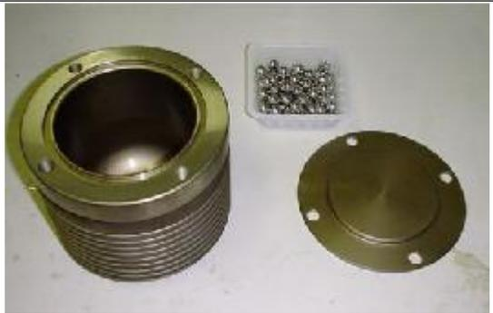
Figure 4: planetary ballmill container, self-made
