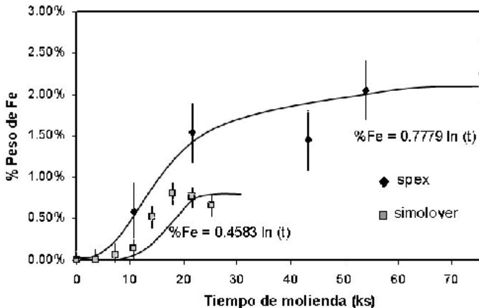
Figure 9: Fe-contamination by microanalysis
