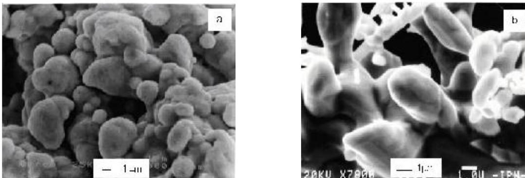
Figure 6: SEM-micrographs of the starting powders (a) Cu and (b) Ag
