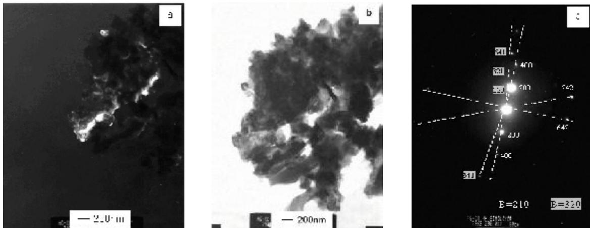
Figure 13: TEM-investigation of the MM powders in the Simoloyer: (a) darkfield micrograph, (b) brightfield micrograph, (c) diffraction pattern after 14.4 ks
