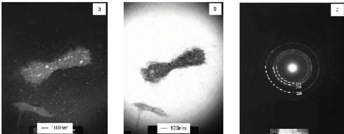
Figure 12: TEM-investigation of the MM powders in the Simoloyer: (a) darkfield micrograph, (b) brightfield micrograph, (c) diffraction pattern after 18.0 ks
