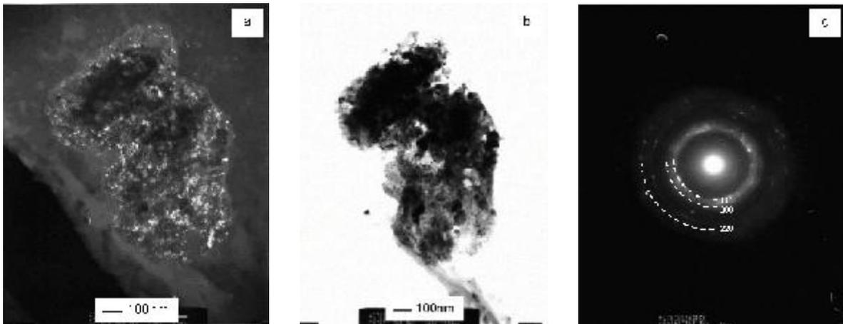
Figure 11: TEM-investigation of the MM powders in the SPEX-mill: (a) darkfield micrograph, (b) brightfield micrograph, (c) diffraction pattern after 43.2 ks
