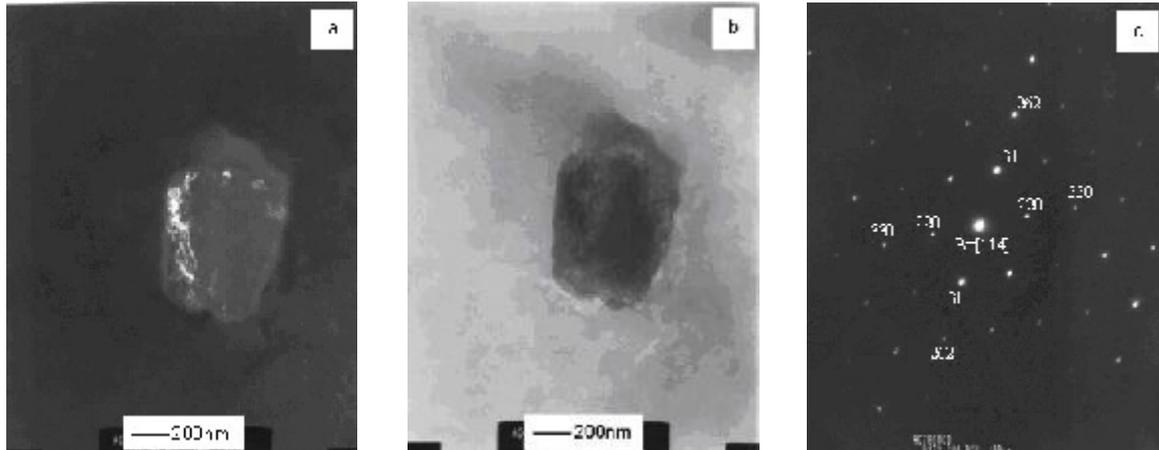
Figure 14: TEM-investigation of the MM powders in the Simoloyer: (a) darkfield micrograph, (b) brightfield micrograph, (c) diffraction pattern after 25.2 ks
