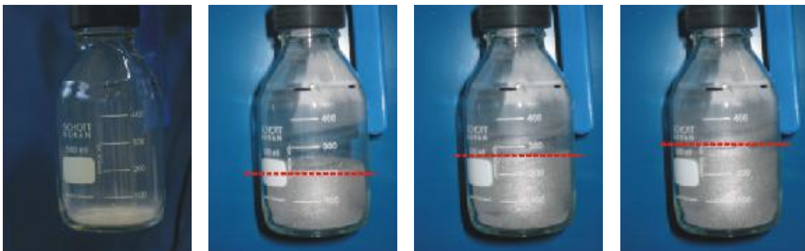
Figure 16: series of pictures for digital measurement of the powder yield at each fix-point
