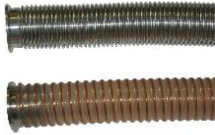
Figure 13: conductive flexible pipes and replaced flex-metal-tubes
