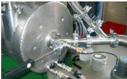
Figure 23: draingrating RD-NW16-DN25 with temperature measurement
