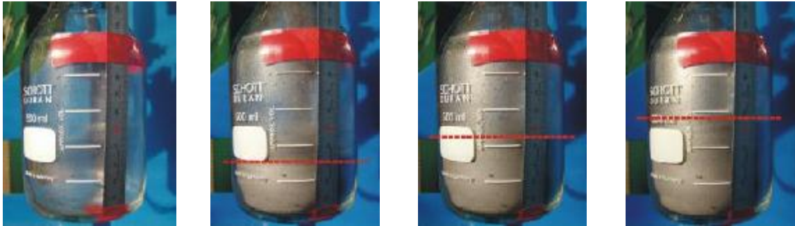
Figure 30: series of pictures for digital measurement of the powder yield at each fix-point
