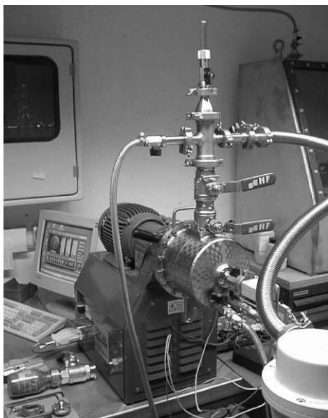
Figure 2: 2-L horizontal high energy ball-mill (Simoloyer CM01-21) with vacuum and inert-gas loading, operation and unloading.
