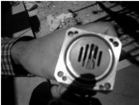
Figure 15: broken center-edge of draingrating, dimensional improvement is recommended
