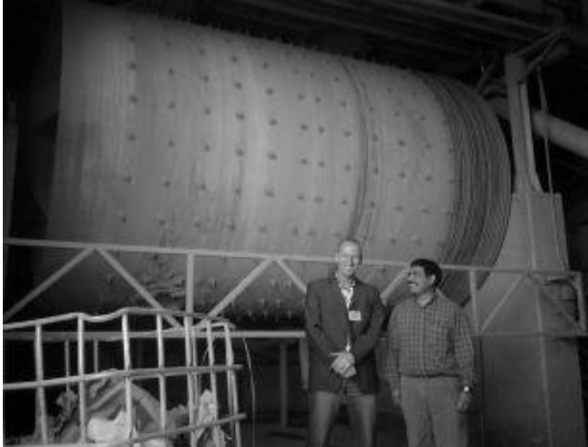
Figure 17: huge drum(ball)mill at Interceramic in Chihuahua, Mexico
