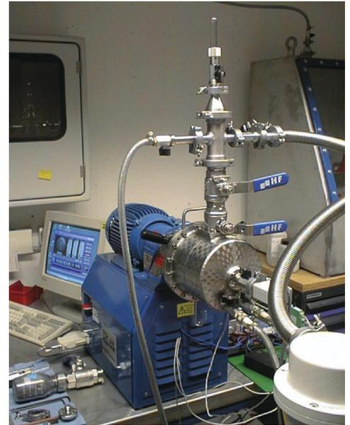
**Fig. 2: horizontal rotary ball mill (Simoloyer® CM01-2I) with air-lock for loading, operation and unloading under vacuum and/or inert-gas.**
