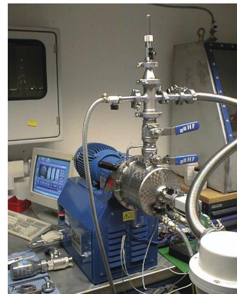
**Fig. 2:** horizontal rotary ball mill (Simoloyer® CM01-21) with air-lock for loading, operation and unloading under vacuum and/or inert-gas.
