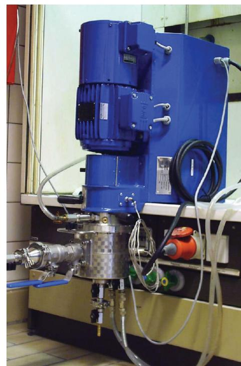
**Fig. 3: Simoloyer® CM01-2l in vertical mount for the leaching process**
