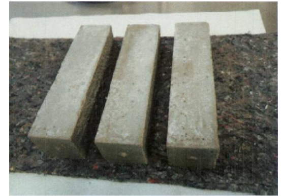
standard prisms 40x40x160 mm 3
