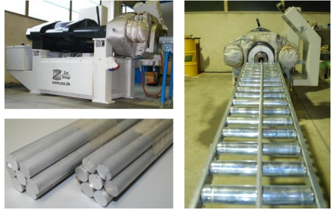
Fig. 2. Hot extrusion of Zentallium ® Z21 to semi-finished products ( here: rods ).
