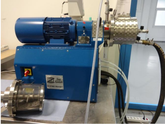
Fig. 1. Simoloyer ® CM01-2lm high energy rotary ball mill and transparent grinding unit (front)
