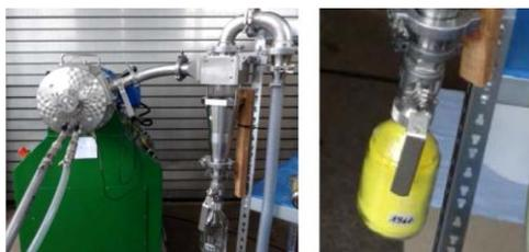
Fig. 4. Provisional open cyclone equipment, collected powder in discharging container after the cyclone.
