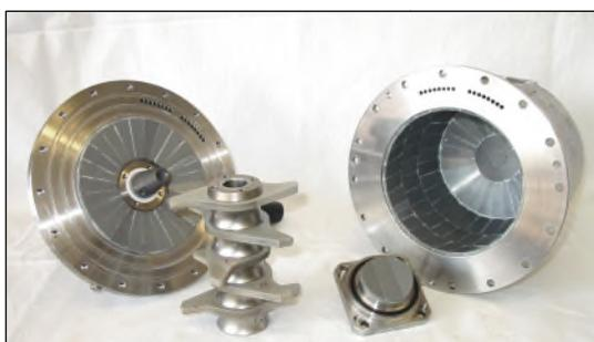
grinding unit W01-2I-SiN disassembled
