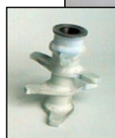
alumina coated rotor
