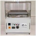
Rollermill RM1s in 4-roll-operation mode (2 driven, 2 non-driven rolls);
