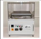
Rollermill RM1s in 4-roll-operation mode (2 driven, 2 non-driven rolls);
