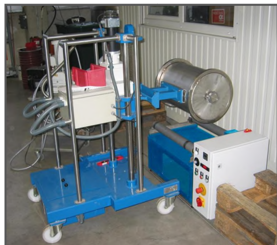
Roller-Mill RM20, during loading with passivation container Zoz-RBP50, still assembled at Container-Track, Zoz-DV63-01
