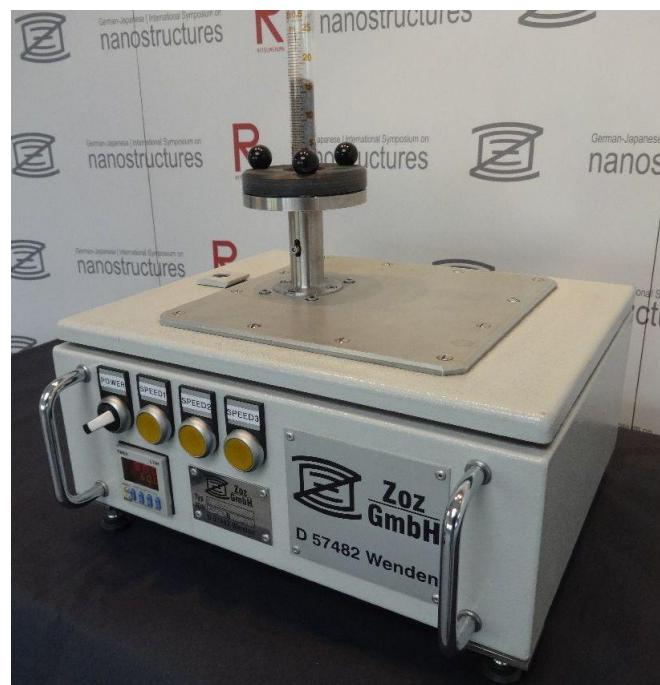
Tap-Densitometer KDM01 with test-cylinders 25 & 100ml
