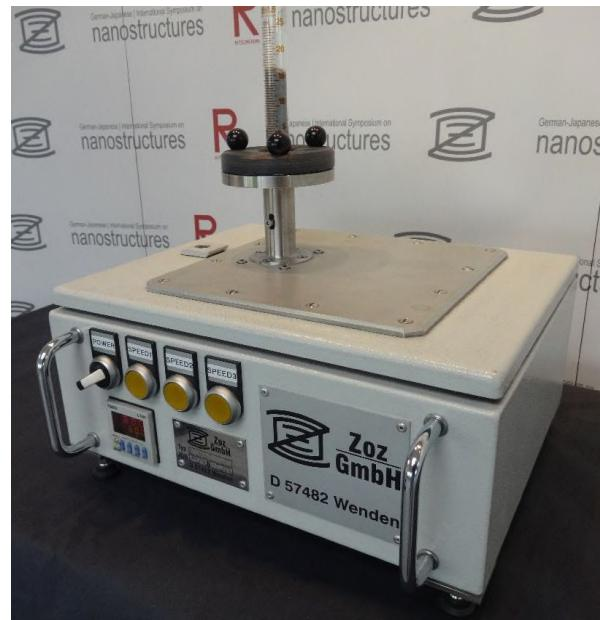
Tap-Densitometer KDM01 with test-cylinders 25 & 100ml
