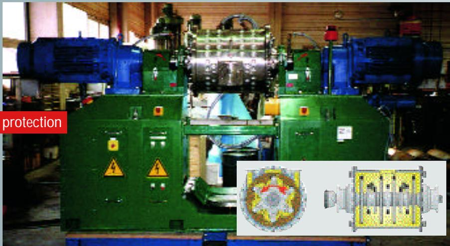
Production unit with a 100 liter chamber. The cross sections through the grinding chamber visualize the working principle. The rotor is the tool to transfer the kinetic energy into the grinding media and these transfer further into the powder materials.
