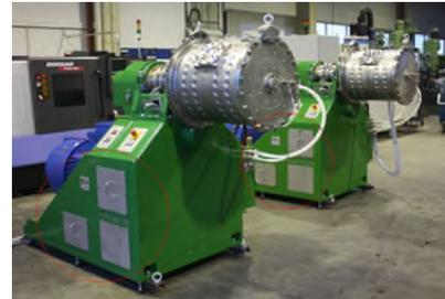
Fig. 1c: CM100, e.g. for production of nanocrystalline metal-hydrides
