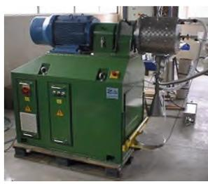
Fig. 1b: CM20, e.g. for production of nano-SiC composites at Zoz
