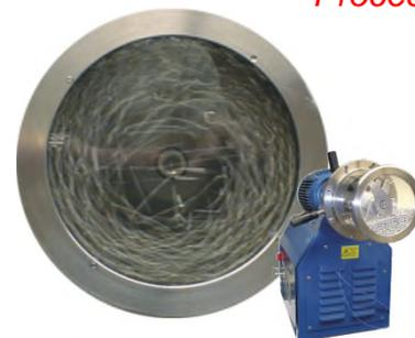
Fig. 5b: Simoloyer<sup>®</sup> CM01 with transparent vessel 01-21
