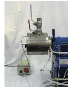
Fig. 12c: heat-able grinding unit & control unit at CM01
