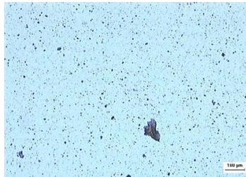
optical micrograph of GCC-HPPC cement powder (processed under the code m60-40-500)
