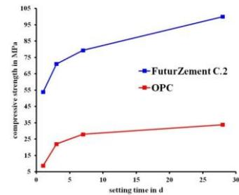
compressive strength: FuturZement C.2 provides 3x higher final strength and 6x higher initial strength than OPC
