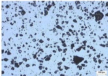
optical micrograph of GCC-OPC cement powder (as received)
