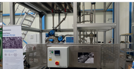
H2-tank B4S-SM in front of Simoloyer® CM100-s2, the Metal-Hydride processing unit (Helmholtz - HZG)
