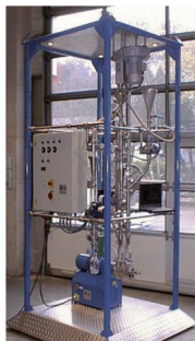
Simoloyer® CM01-20m-s1, lab-scale
