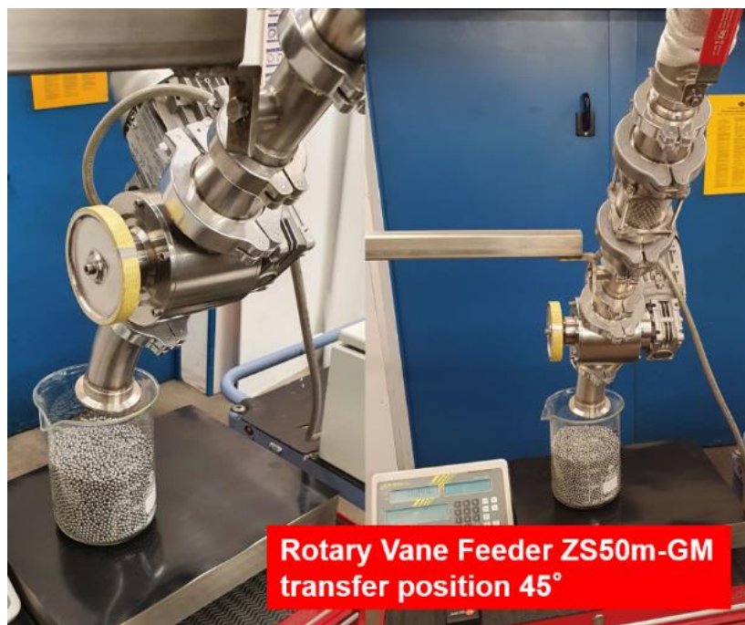
[6a] test configuration 45°, ZS50m-G06, feed-wheel STS-01
