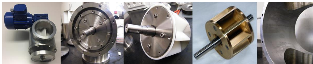
[4] star-feeders 37ZS50.ZR1 utilized in Zoz ZS Rotary Vane Feeders, adjusted mainly in material, seals & surface, in geometry only slightly
