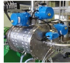
[1b] draining gratings Ask100 (left) and Askm100 (charging) & Bskm100 (discharging) at Simoloyer® CM100 auto-batch (on right)
