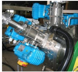
[1a] draining gratings Ask0820 (left) and Askm0820 (charging) & Bskm0820 (discharging) at Simoloyer® CM20 auto-batch (on right)
