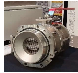
[1b] draining gratings Ask100 (left) and Askm100 (charging) & Bskm100 (discharging) at Simoloyer® CM100 auto-batch (on right)
