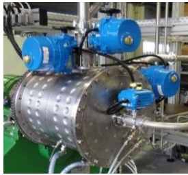
[1a] draining gratings Ask0820 (left) and Askm0820 (charging) & Bskm0820 (discharging) at Simoloyer® CM20 auto-batch (on right)
