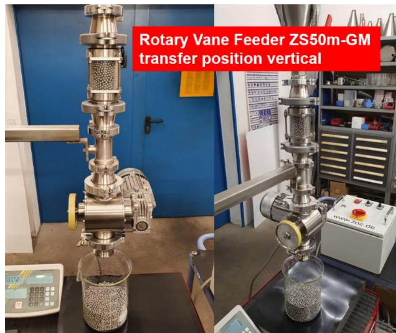
[6b] test configuration 90°, ZS50m-G06, feed-wheel STS-02
