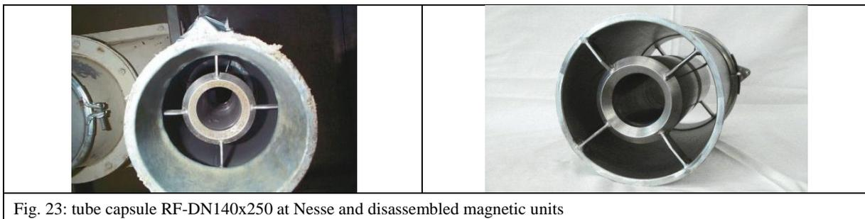
Fig. 23: tube capsule RF-DN140x250 at Nesse and disassembled magnetic units
