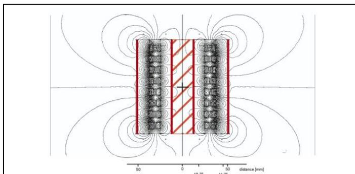
Fig. 11: chart of magnetic flux lines of magnetic filter MF-DN100x110
