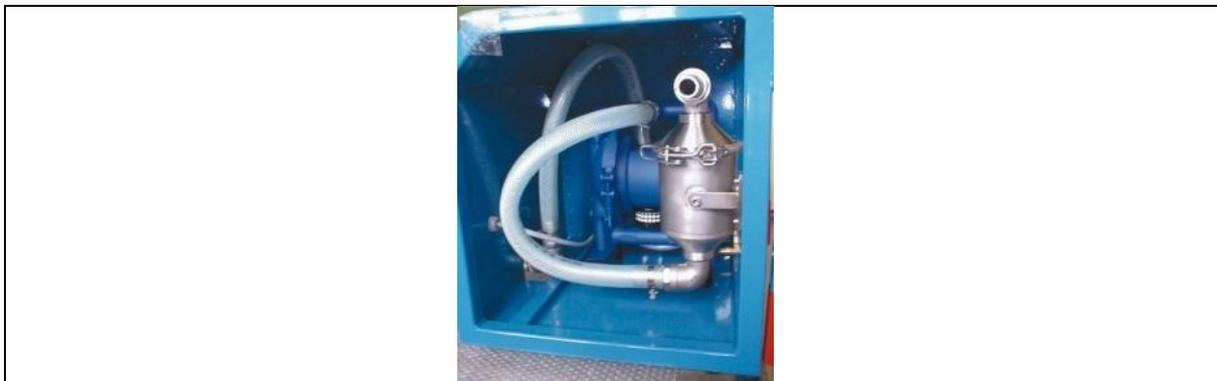
Fig. 20: pressure capsule D-MF1011\*with assembled magnetic filter in a pump-line at a Zoz-screen-cart
