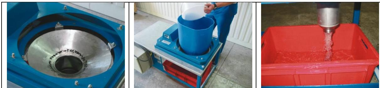
Fig. 13: experimental set up for Fe-powder and water, simulation of full water flow, water drained
