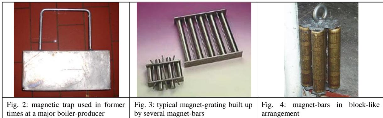
A somewhat more sophisticated technically route is to build up a barrier for a volume flow of product in order to force it passing close to the magnet surface. However, the main problem is defined by the word *barrier* already. In order to have an acceptable barrier, its design leads usually to a non-barrier.
