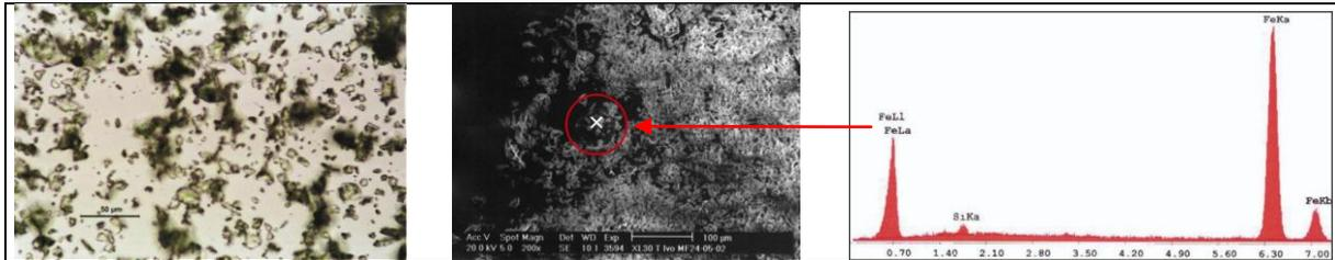
Fig. 19: optical microscopy, SEM and EDX Analysis of separated particles, very high Fe-content
