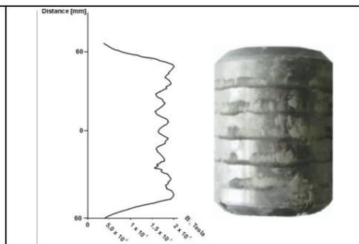
Fig. 12: magnetic flux density at air induction at res. of magnetic unit MK-078105
