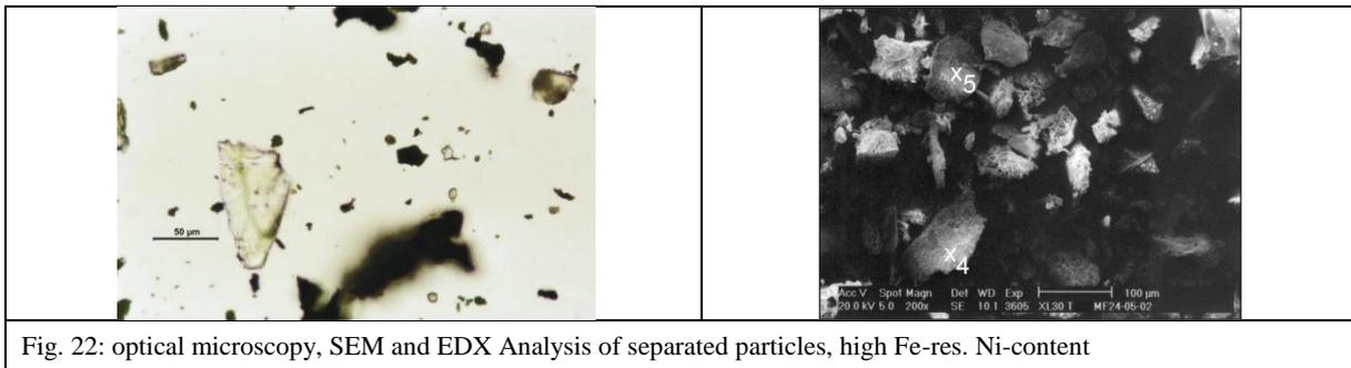
Fig. 22: optical microscopy, SEM and EDX Analysis of separated particles, high Fe-res. Ni-content
