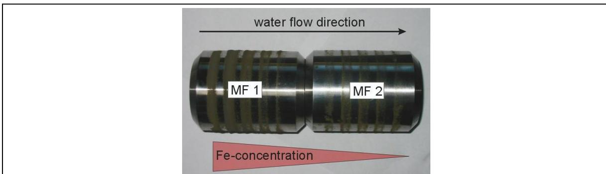
Fig. 16: the 2 magnetic units as dismantled after the test of Fe-powder and water
