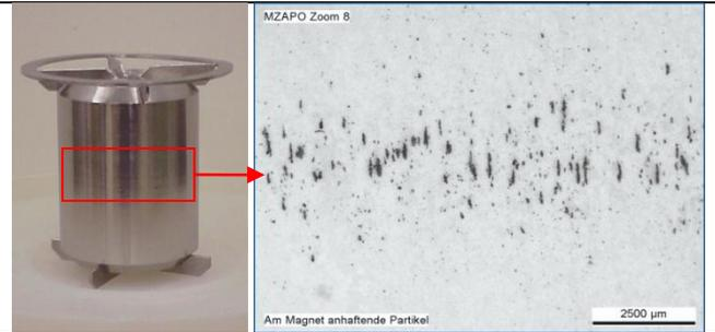
Fig. 18: separated waste on the outer surface of the magnetic unit and enlarged
