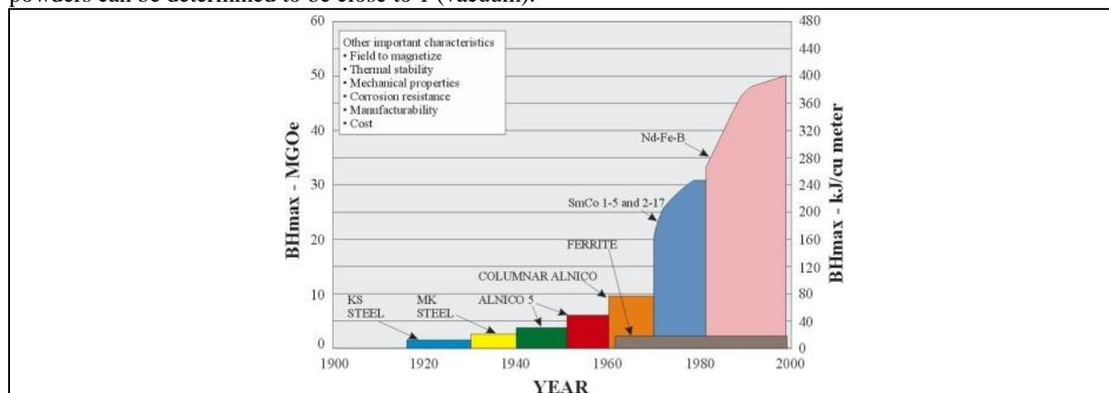
Fig. 10: Development of Permanent Magnets in the 1900's
