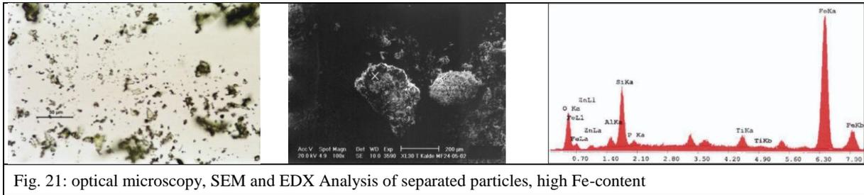
Fig. 21: optical microscopy, SEM and EDX Analysis of separated particles, high Fe-content
