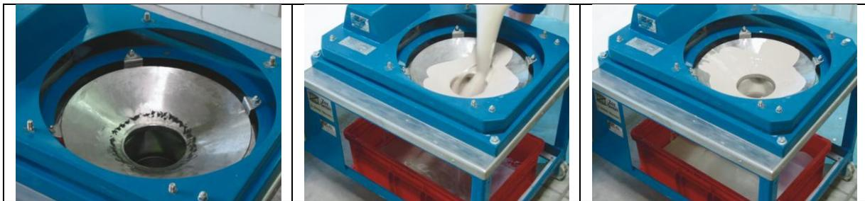
Fig. 15: experimental set up for Fe-powder and enamel slurry, simulation of full slurry flow, enamel slurry drained
