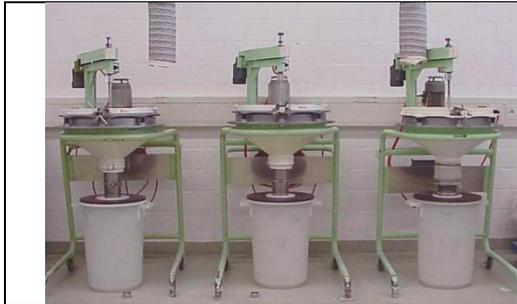
Fig. 17: 3 / 6 sieving operations at Ivoclar Vivadent with ea. 2 adapted magnetic filters MF-DN100x110
