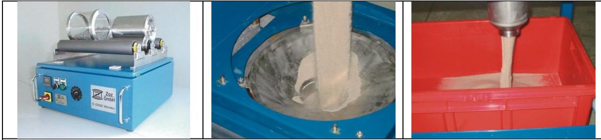
Fig. 14: mixing of Fe-powder in sand in a Zoz-Rollermill RM1, simulation of full powder flow, sand drained
