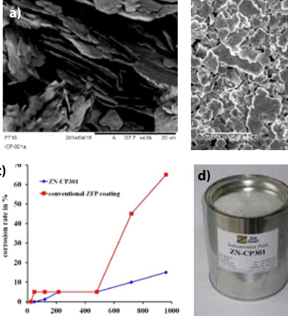
**Fig. 10a-d:** HKP-ZFP (Zinc-Flake by Simoloyer®), a) SEM), b) corresponding Zn-lamellar layer, c) corrosion rate of ZN-CP301 vs. conventional ZFP coating at salt spray test and d) a product can of anticorrosive paint ZN-CP301
