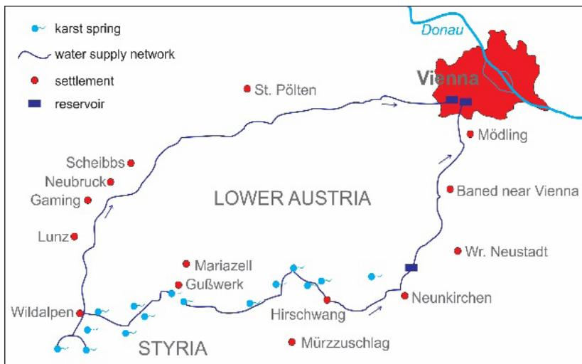
**Fig. 4:** Vienna is supplied with drinking water from karst springs nearly 200 km away via two long-distance mains (Source: Vienna's Water Supply, 2016).
