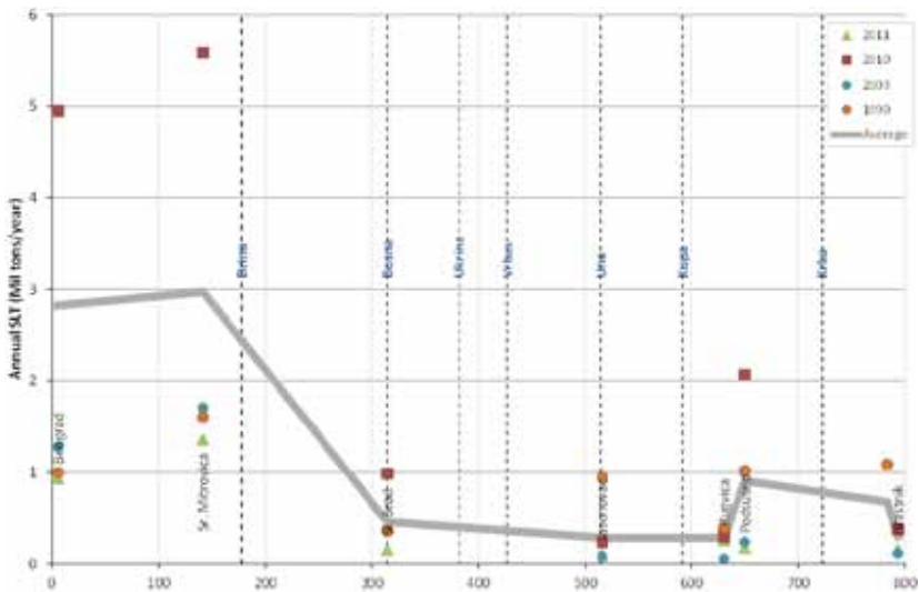
**Fig. 7:** The longitudinal presentation of the annual suspended sediment loads along the Sava River in selected years (ISRBC, 2013; Fig. 56, p. 62).
