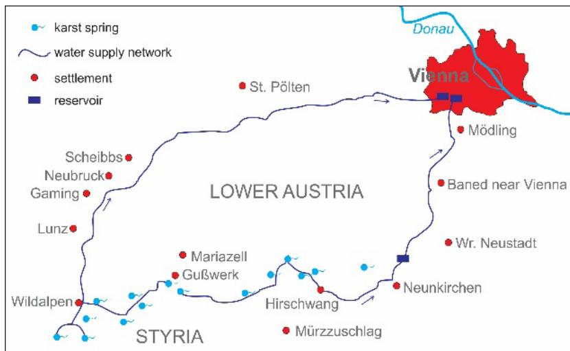
**Fig. 4:** Vienna is supplied with drinking water from karst springs nearly 200 km away via two long-distance mains
