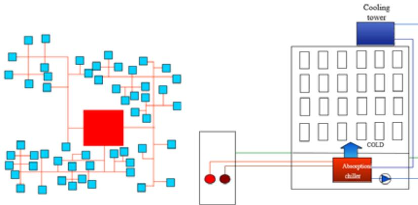
**Fig. 8:** District cooling system with local cold production
