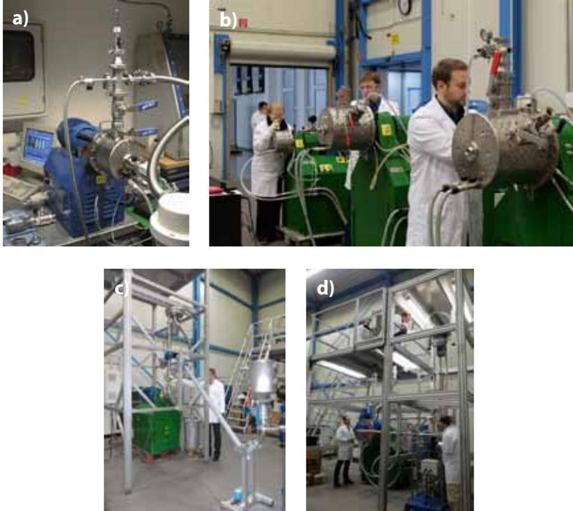
**Fig. 1:** a) Simoloyer® CM01-2lm laboratory scale with air-lock, b) Simoloyer® CM08lm (back) and CM20lm in front, c) Simoloyer® CM20-20lm-s1 semi continuous operation mode and d) Simoloyer® CM100-s2, auto-batch operation mode
