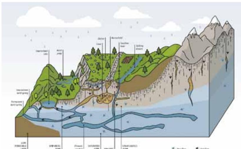
**Fig. 7:** Schematic illustration of a typical karst landscape and its hydrological characteristics (Ravbar & Šebela 2015).
