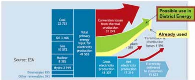
2/3 of the fuel is converted to heat energy and could be used for heating and cooling
