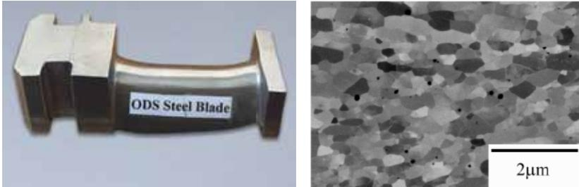
**Fig. 11:** turbine blade from ODS steel (picture taken from Zoz-ARCI Center, India) and BSE SEM image of 14 YWT (DiDomizio 2014)
