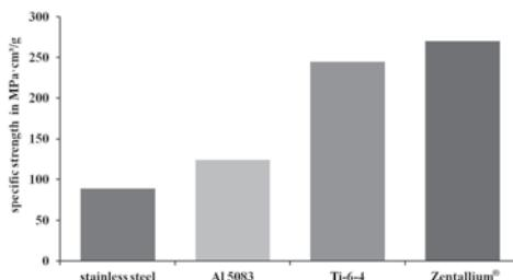
**Fig. 5:** specific strength of stainless steel, Al- and Ti- alloys and Zentallium®
