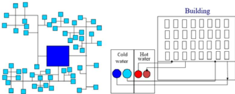
Cold distribution: water, water solution, ice slurry
