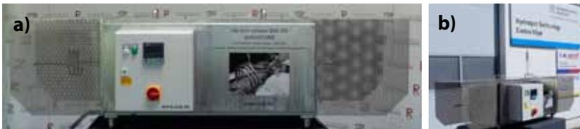
**Fig. 9:** a) H<sub>2</sub>-tank system B4S-SM complex metal hydrides and b) HZG@ZTC
