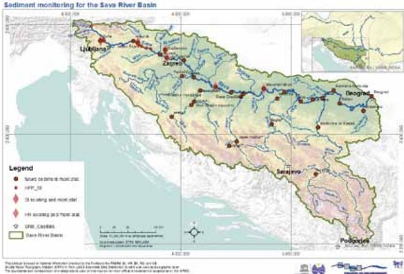
**Fig. 10:** *The sediment monitoring in the SRB (ISRBC, 2015; p. 49) – showing the existing and the proposed future sediment monitoring stations on the Sava River and its tributaries.*
