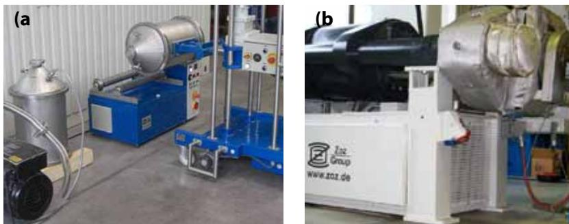
**Fig. 2a-b:** Passivation of Zentallium® powder after Simoloyer® – processing and hot extrusion at ZTC
