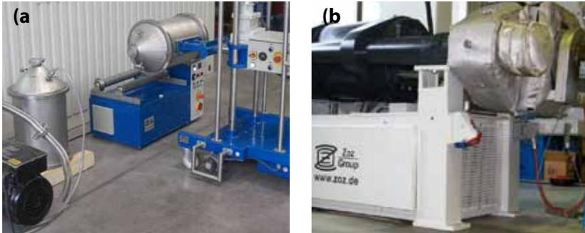
**Fig. 2a-b:** Passivation of Zentallium® powder after Simoloyer® – processing and hot extrusion at ZTC
