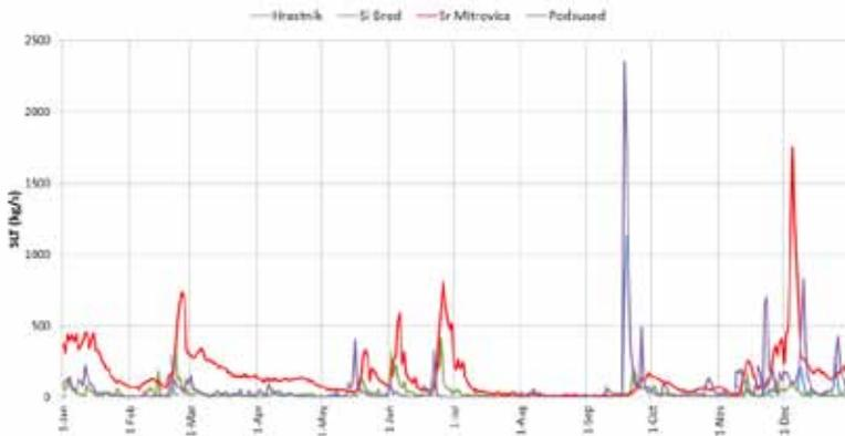
**Fig. 8:** Daily suspended sediment loads along the Sava River in 2010 (ISRBC, 2013; Fig. 60, p. 65).
