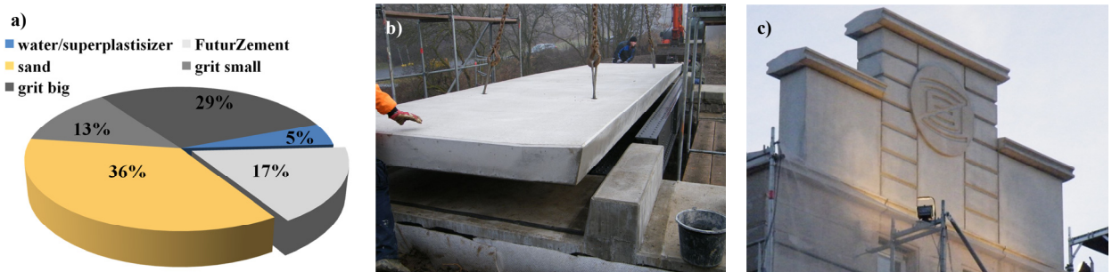
Fig. 6. a) Composition of FuturBeton, b) concrete slab of public bridge “Rosenthal” (est. November 2012) and c) roof façade at “Villa ZCS” (est. June 2013).
