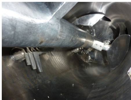
Fig. 5. Inside plough-share mixer with milling heads.
