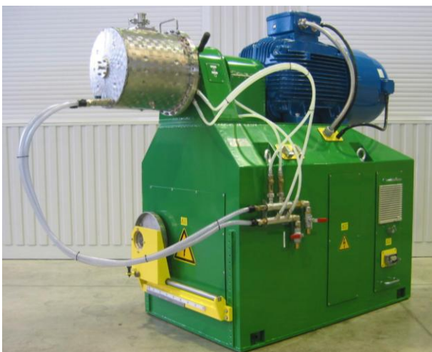
Fig. 3. Simoloyer ® CM20-20lm high energy ball mill This technique can be scaled-up from laboratory
