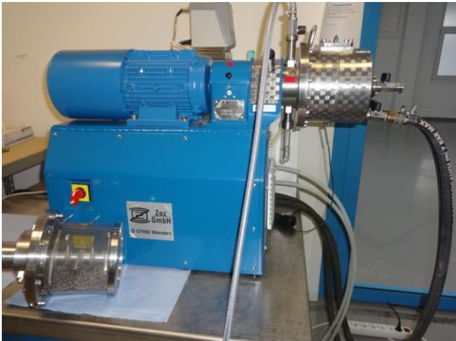
Fig. 1. Simoloyer<sup>®</sup> CM01-2lm high energy rotary ball mill and transparent grinding unit (front)
