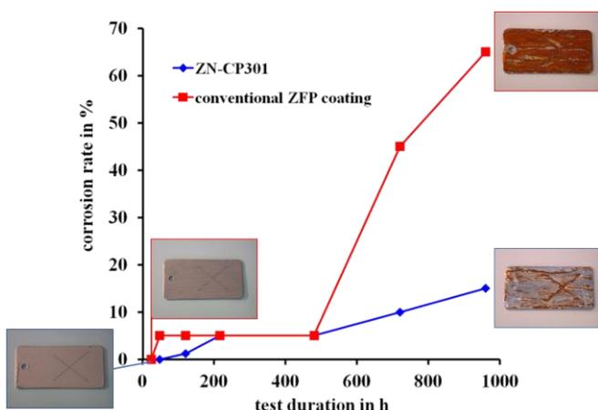
Fig. 5. Corrosion protection of ZN-CP301 and conventional zinc flake coating in salt spray test.
