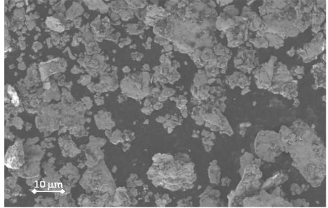
Fig. 2. Zinc Flakes by High Kinetic Processing
