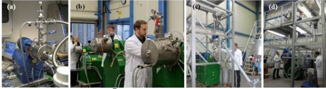
Fig. 1. Simoloyer ® CM01-21m laboratory scale with air-lock (a); Simoloyer ® CM081m (back) and CM201m in front (b); CM201m-s1, semi-continuous operation mode (c) and Simoloyer ® CM100-s2, auto-batch operation mode.
