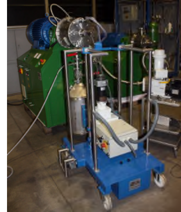
passivation container RBP50 equipped with air-lock DN50KF, gassing-valve and evacuation unit at a container-track/manipulator DV63-01 in front of a Simoloyer CM20 at Al-matrix material manufacturing
