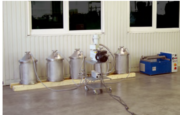
handling of high reactive material: 5 units RBP50 at vacuum-pump station
