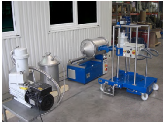
RBP50 placed on a roller-mill RM20 by DV63-01 for controlled passivation of Al-base materials
