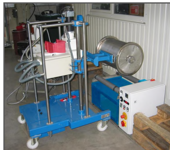
Roller-Mill RM20, during loading with passivation container Zoz-RBP50 still assembled at Contain-Track, Zoz-DV63-01
