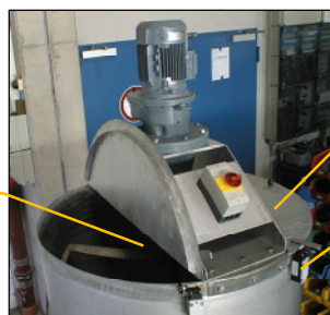
Agitated tank RW10 with options cooling- / heating-jacket and blind lid
