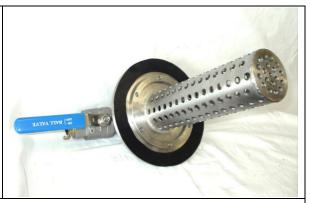
auxiliary pipe and ring nozzle, flat seal customized
