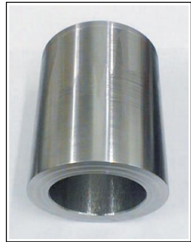
bearing bush – composite system (consolidated PM-Stellite on 1.4404)
