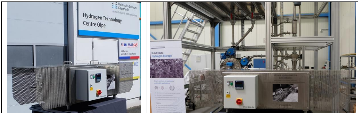
H2-tank system B4S-SM at ZTC in Olpe and inside at the Helmholtz HZG - Hydrogen Technology Centre in front of the Zoz-Simoloyer® CM100-s2, a processing unit for the manufacturing of complex metal hydrides
