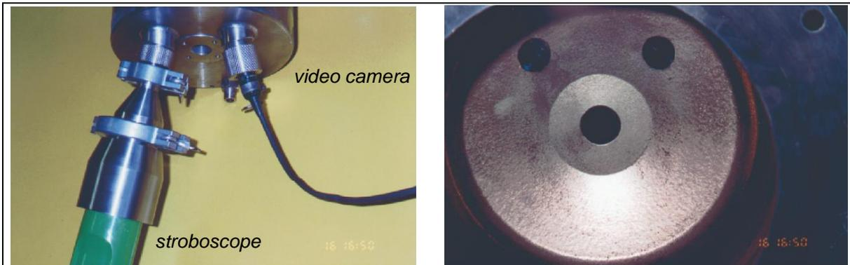
Fig. I-3: grinding unit with video equipment, outside & inside view
