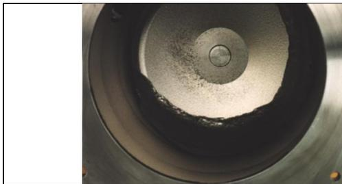
Fig. IV-16: grinding chamber after constant operation
