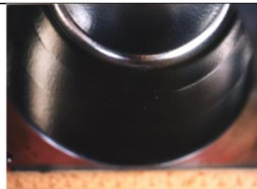
Fig. IV-17: grinding chamber after cycle operation
