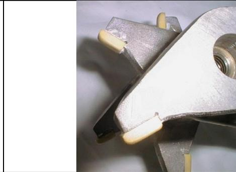
Fig. VII-10: ZrO2 rotor after 1h, the rotor tips worn out
