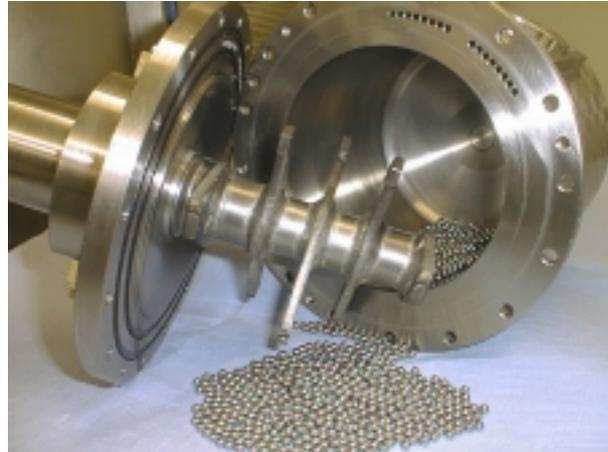
*Fig. 6: Grinding Unit of Simoloyer CM01-2l, grinding media*
