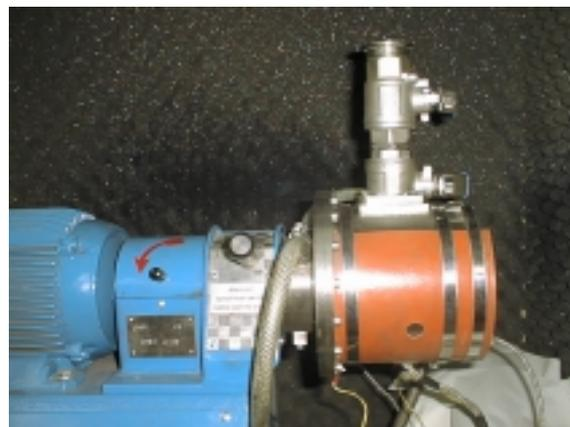
Fig. 5: *Grinding unit with heating element*
