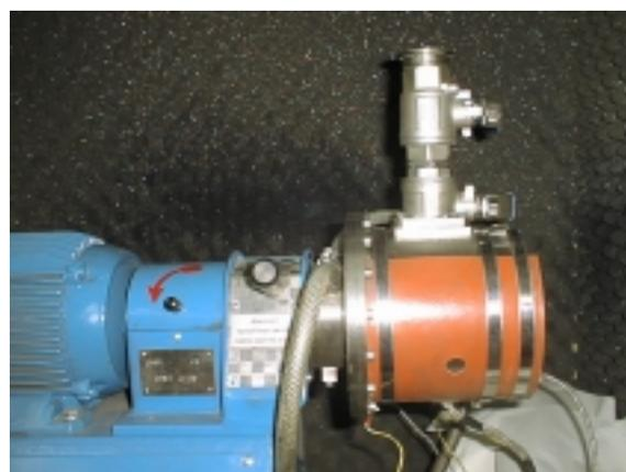
Fig. 5: *Grinding unit with heating element*
