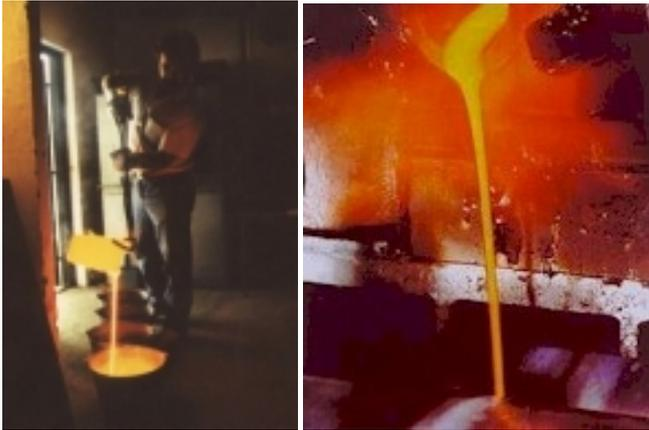
Fig. 03: unloading of a turn-tube-furnace into water-flow (left) and onto cooling roll (right)
