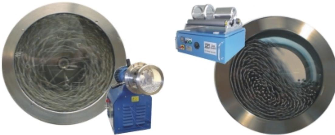
Fig. 08: grinding media motion in (a) a high kinetic system (Simoloyer) and (b) in a low kinetic system (Rollermill RM1)
