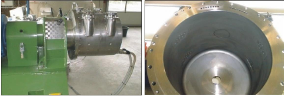
Fig. 24: W20-20ls1, semi-continuously grinding unit with DN40 tangential ports
