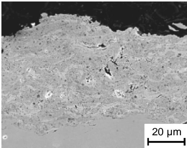
**Figure 6.** Cross section of a Co-based SiC composite coating type 3, SiC content in the composite powder: 65 vol.-%, Top Gun K.
