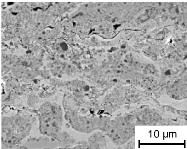
**Figure 7.** SEM detail image of a Co-based SiC composite coating type 3 cross section, SiC content in the composite powder: 65 vol.-%.
