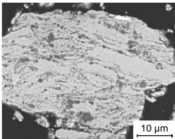
**Figure 3.** SEM image of a powder particle cross section, Ni-based SiC composite matrix type 1, SiC content in the composite powder type 1: 50 vol.-%, Simoloyer CM 01-2l.
