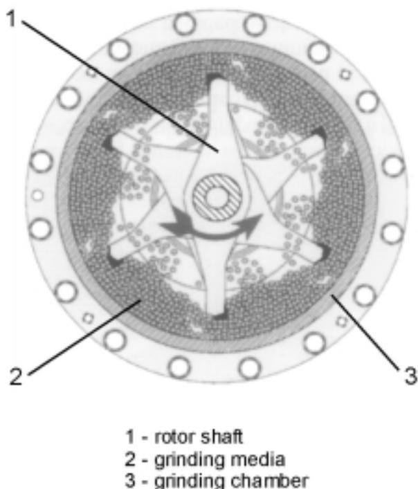
**Figure 1.** Cross-sectional view of the Simoloyer grinding unit with horizontal rotor shaft, milling balls and grinding chamber
