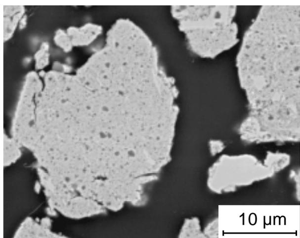
**Figure 4.** SEM image of a powder particle cross section, Co-based SiC composite matrix type 3, SiC content in the composite powder: 70 vol.-%, Simoloyer CM 08-08l.
