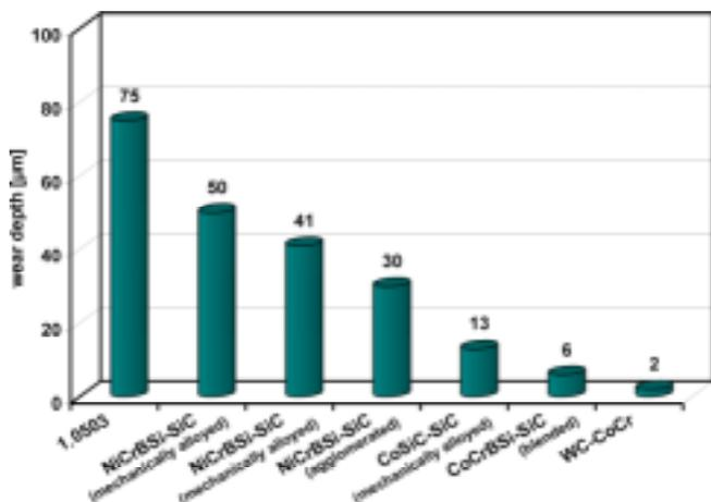
**Figure 9.** Oscillating wear test results of the nano-structured SiC-composites.
