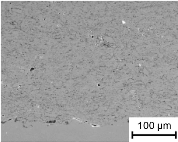
**Figure 5.** Cross section of a Ni-based SiC composite coating type 1, SiC content in the composite powder: 50 vol.-%, Diamond Jet Standard.
