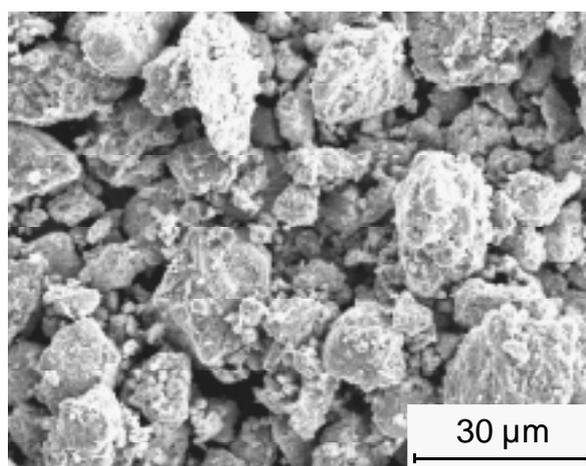
**Figure 2.** Morphology of the mechanically alloyed composite particles.
