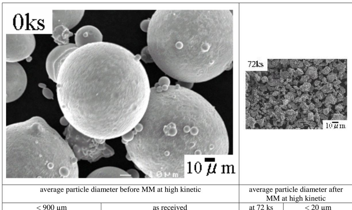
Figure 9: SEM of MM-powder after 0 and 72 ks at high kinetic (CM01)
