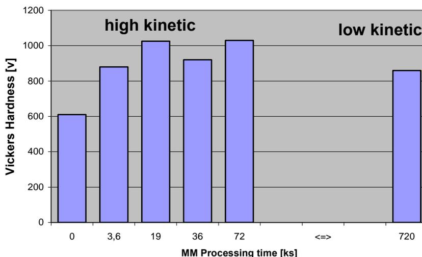
Figure 15: Vickers hardness test of SPS-samples consolidated from the MM-powders
