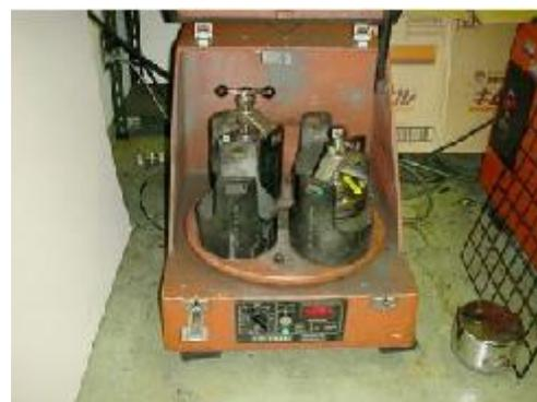
Figure 3b: planetary ballmill Fritsch P-5
