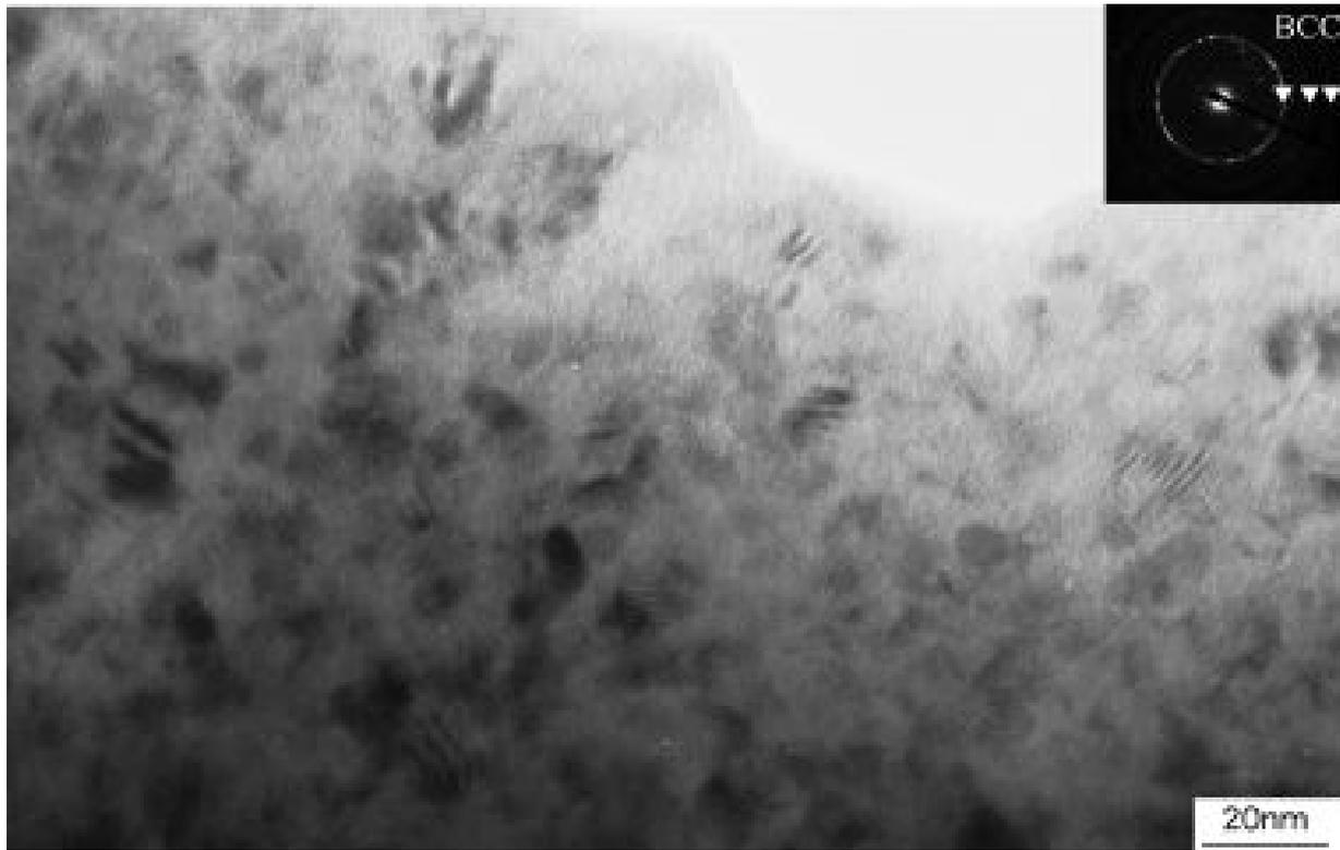
Figure 2: TEM bright field analysis of MM-HSS powder identified in table 1.
