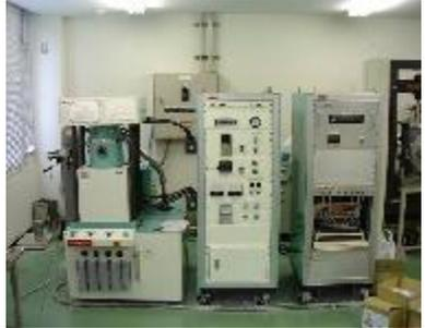
Figure 6: Electrical Discharge (Spark) Plasma Sintering device
