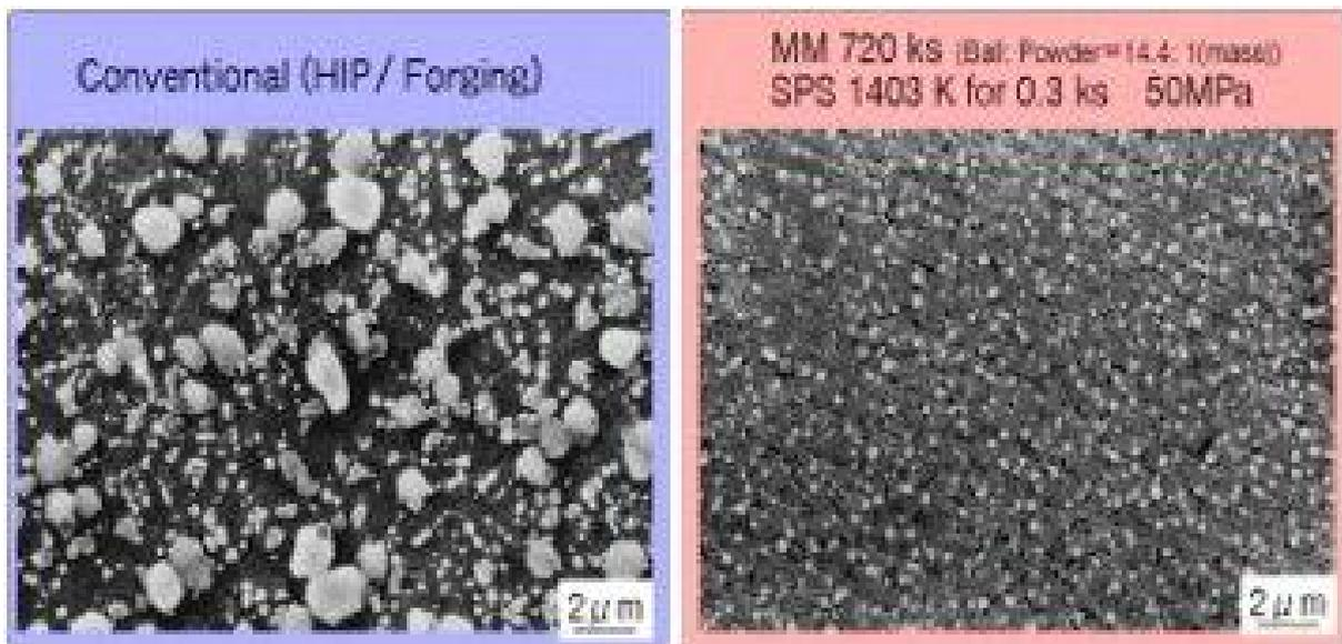
Figure 17a-b: SEM of conventional HSS-compact by HIP/Forging and of MM/SPS compact
